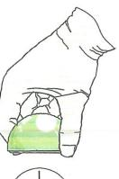
2. Push the Self-Aligning Acetabular Cup onto the Bearing until the metallic snap ring on the bearing engages the groove in the Cup. Be sure to align the metal cup with the metal ring evenly before seating the metal shell.
